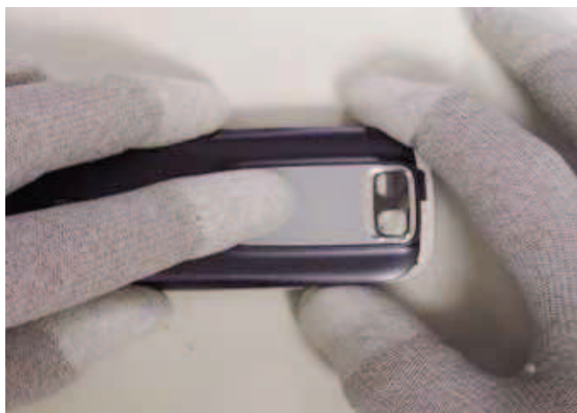
1) Slide the battery cover down.
