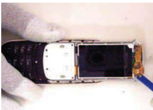
13) Use the SS-93 to remove the LCD connector.
