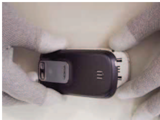
2) Lift and remove the battery cover.
