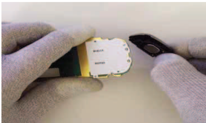
25) Remove the antenna assy.
