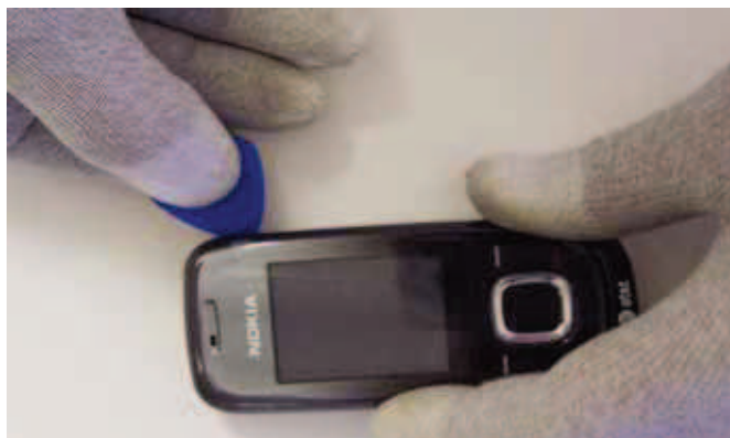
5) Slide the SRT-6 along the sides to release the tabs.
