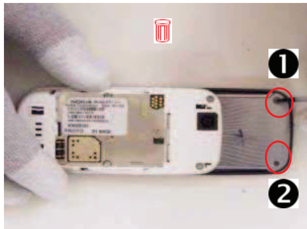
4) Use the #4 TORX screwdriver to remove the 2 screws in the order shown. Discard the screws.
