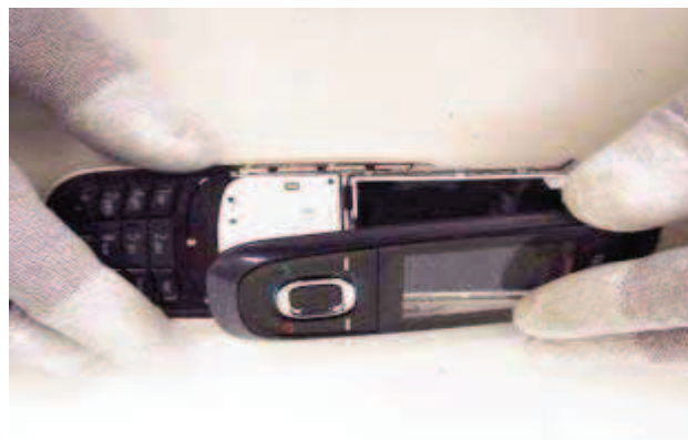
6) Lift and remove the A-Cover.
