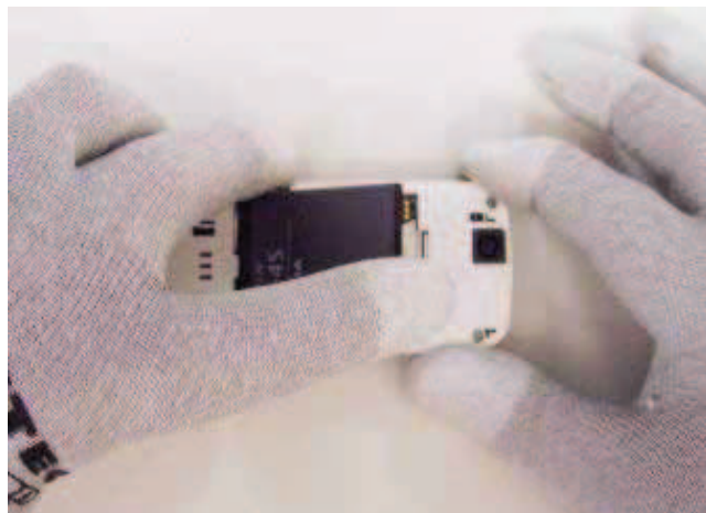
3) Lift and remove the battery.
