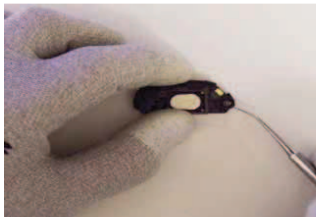
26) Use the dental pick to remove the mic.
